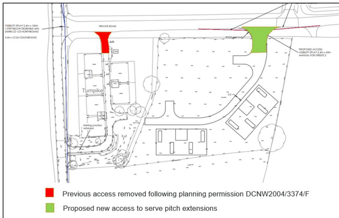
Figure Two: Plan comparing previous and proposed access arrangements to Torvale Road
